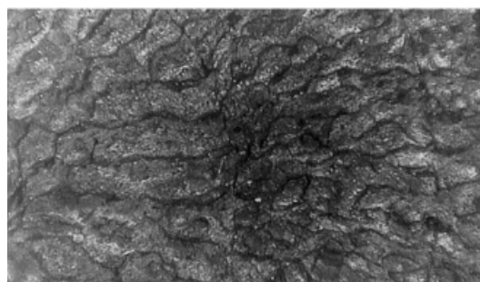
Figure 17 Top view of worn surface of filled NR compound, showing abrasion pattern (normal load = 25 N; magnification = \times 40 ). (A) without ground rubber powder (wear rate = 0.21 mg/rev; 100% modulus = 22 kg/cm 2 ; pattern spacing = 0.8 mm); (B) with ground rubber powder (particle size = 420–600 \mu\text{m} ; loading = 50 phr; wear rate = 0.17 mg/rev; 100% modulus = 30 kg/cm 2 ; pattern spacing = 0.5 mm).
